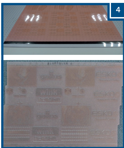
Cut printing plate on Kongsberg table.
