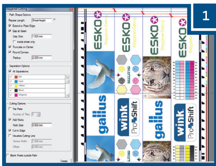
Make Step & Repeat in Plato or ArtPro Powerstepper , select „Staggered Cutting“ dialogue box and automatic drawing tool.
