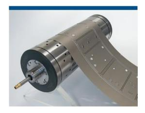
The wink **FlexAir** system combines the advantages of solid die air systems with those of flexible dies. Air passage holes on the surface of the **FlexAir** magnetic cylinder align exactly with the holes in the corresponding flexible die so that the cut-out waste can be blown directly into the extraction unit which is attached to the vacuum system.
